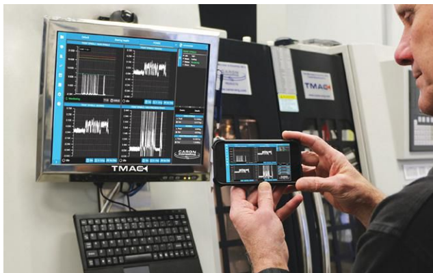
Caron Engineering’s TMAC system can display multiple sensor channels at the same time, even on a handheld device. (Provided by Caron Engineering)
