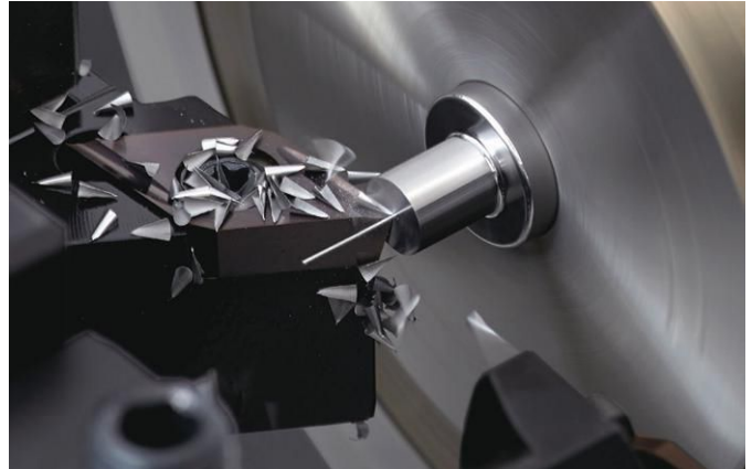
Citizen's low-frequency vibration technology oscillates the Z axis while cutting to consistently break chips. (Provided by Marubeni Citizen-Cincom)
