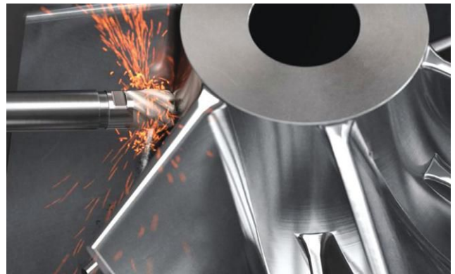
Solid round ceramic tools (here from Sandvik Coromant) are emerging as a solution for some challenging aerospace applications like this blisk. (Provided by Sandvik Coromant)
